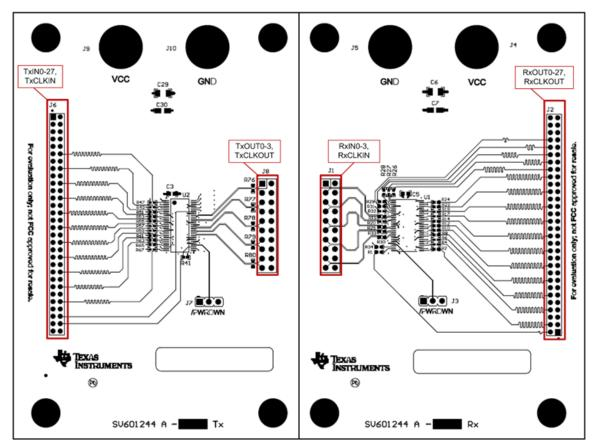
Figure 2. DS90CR285-86ATQEVM Input and Output Pins
