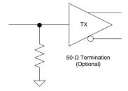
Figure 4. Schematic of Optional Parallel Input 50-Ω Termination to GND
