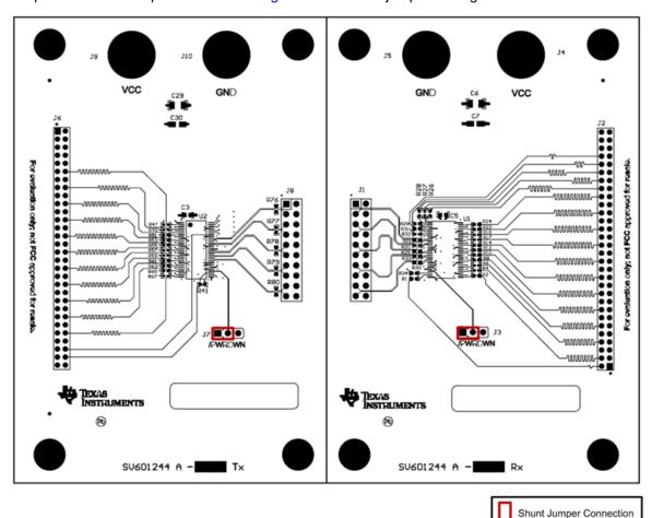
Figure 6. DS90CR285-86ATQEVM Default Jumper Pin Settings
