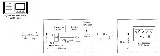
Figure 8. Typical Test Setup With Generator and Scope
