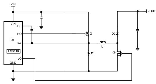
Figure 1. Two Switch Simplified Block Diagram
