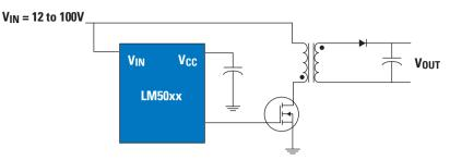
Figure 2a: PWM IC running off a high input voltage in a low power system
