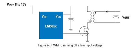
If the input voltage lies between 8 and 15V, the LM50xx controllers are particularly easy to power. The  $V_{IN}$  and  $V_{CC}$  pins can simply be tied together and to the input voltage, which then directly powers the controller. (*Figure 2c*). If the voltage exceeds 15V the two pins cannot be tied together, and the input voltage has to be higher than about 12V in order for the controller to start up.
