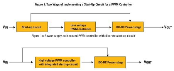
Figure 1b: Power supply built around PWM controller with integrated start-up circuit
