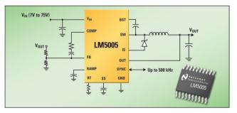
The LM5005 is available in a power enhanced TSSOP-20 package featuring an exposed die attach pad to aid thermal dissipation. It is ideal for use in consumer electronics, telecommunications, data communications systems, automotive power systems, and distributed power applications.
