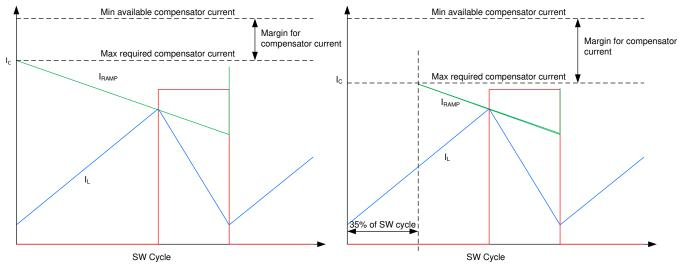
Figure 1. Boost I<sub>RAMP</sub> Delay Function
