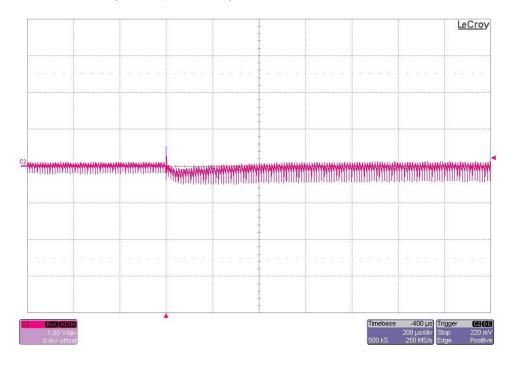
The photo below shows the 120V output voltage (ac coupled) when the load current is stepped from 10mA to 5mA. Vin = 36Vdc (1V/DIV, 200uS/DIV)
