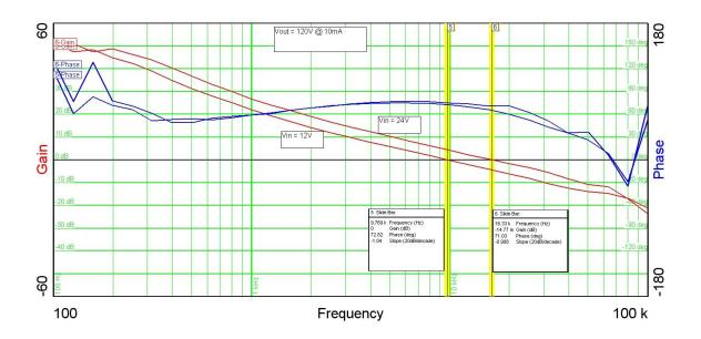
The plot below shows the loop gain with the input voltage at 12V and 24V with the output loaded to 5mA.
