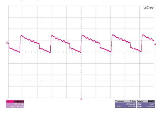
The 120V output ripple voltage is shown in the figure below. The image was taken with the output loaded to 10mA and the input voltage set to 12Vdc. (200mV/DIV, 5uS/DIV)
