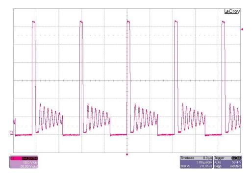
The photo below is the N-ch FET (Q1) drain waveform. The input voltage is 12V and the output is loaded to 10mA. (10V/DIV, 5uS/DIV)
