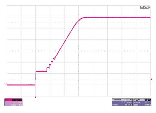
The photo below shows the 120V output voltage startup waveforms after the application of 24Vdc in. The output was loaded with a 10mA load. (20V/DIV, 5mS/DIV)
