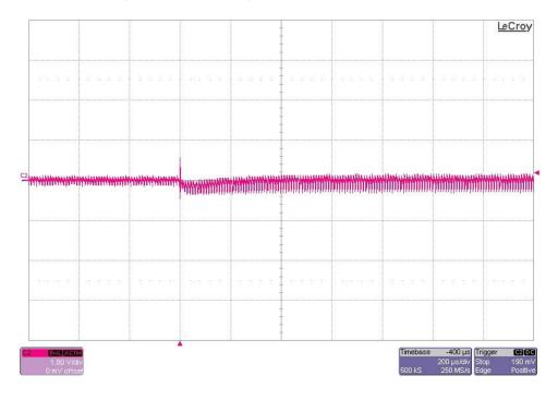
The photo below shows the 120V output voltage (ac coupled) when the load current is stepped from 10mA to 5mA. Vin = 12Vdc (1V/DIV, 200uS/DIV)
