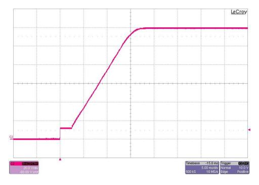
The photo below shows the 120V output voltage startup waveforms after the application of 12Vdc in. The output was loaded with a 10mA load. (20V/DIV, 5mS/DIV)
