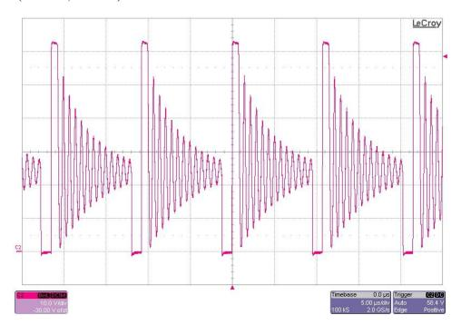
The photo below is the N-ch FET (Q1) drain waveform. The input voltage is 36V and the output is loaded to 10mA. (10V/DIV, 5uS/DIV)
