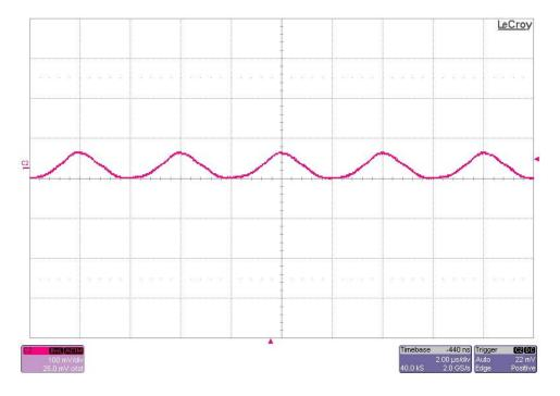
The 24V output ripple voltage (AC coupled) is shown in the figure below. The image was taken with the output loaded to 2A. The input voltage is set to 60V. (100mV/DIV, 2uS/DIV)
