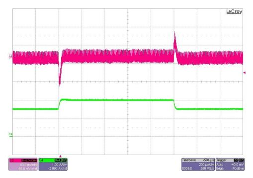
The photo below shows the output voltage (ac coupled) when the load current is stepped between 1A and 2A. Vin = 28V. (100mV/DIV, 1A/DIV, 200uS/DIV)
