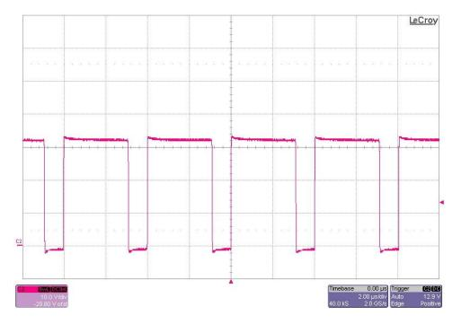
The photo below shows the FET switching voltage. The input voltage is 60V and the output is loaded to 2A. (10V/DIV, 2uS/DIV)
