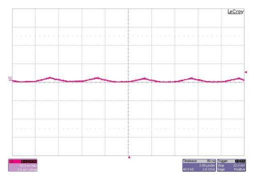
The 24V output ripple voltage (AC coupled) is shown in the figure below. The image was taken with the output loaded to 2A. The input voltage is set to 28V. (50mV/DIV, 2uS/DIV)
