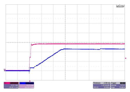
The photo below shows the output voltage startup waveform after the application of 28V in. The 24V output was loaded to 2A. (10V/DIV, 1mS/DIV)
