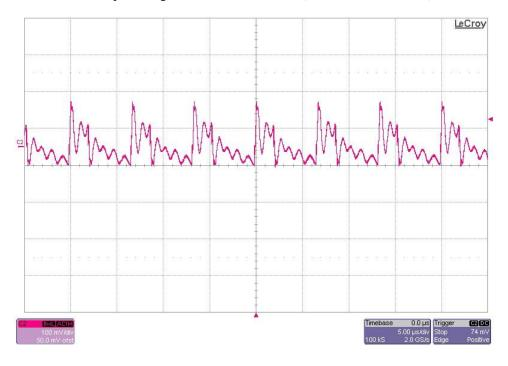
The 13.2V output ripple voltage (AC coupled) is shown in the figure below. The image was taken with the output loaded to 3A. The input voltage is set to 16V. (100mV/DIV, 5uS/DIV)
