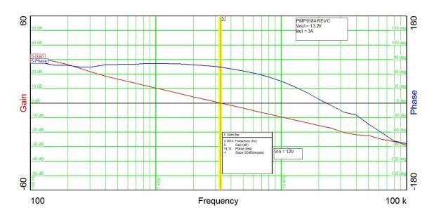
The plot below shows the loop gain with the input voltage set to 12V and the output set to 1A.
