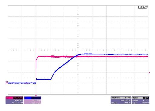
The photo below shows the output voltage startup waveform after the application of 12V in. The 13.2V output was loaded to 3A. (5V/DIV, 5mS/DIV)
