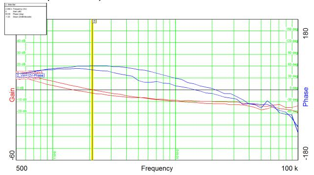
$\begin{array}{ll} \text{Output power} & = 51 \text{V}@1.25 \text{A} \\ \text{Input voltage} & = 9 \text{VDC} \\ \text{Phase margin} & = 54^{\circ} \\ \text{Bandwidth} & = 1.5 \text{kHz} \end{array}$
