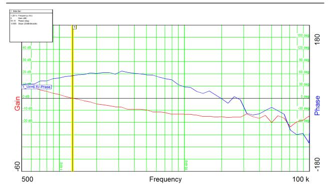
Output power = 51V@0.5AInput voltage = 6.5VDCPhase margin  $= 55^{\circ}$ Bandwidth = 1.3kHz
