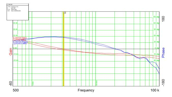
$\begin{array}{ll} \text{Output power} & = 51 \text{V}@1.25 \text{A} \\ \text{Input voltage} & = 9 \text{VDC} \\ \text{Phase margin} & = 57^{\circ} \\ \text{Bandwidth} & = 2.4 \text{kHz} \end{array}$
