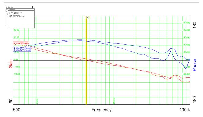
Output power = 51V@1.25AInput voltage = 24VDCPhase margin  $= 79^{\circ}$ Bandwidth = 4.5kHz
