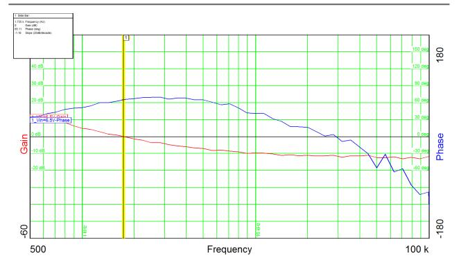
Output power = 51V@0.5AInput voltage = 6.5VDCPhase margin  $= 65^{\circ}$ Bandwidth = 1.7kHz
