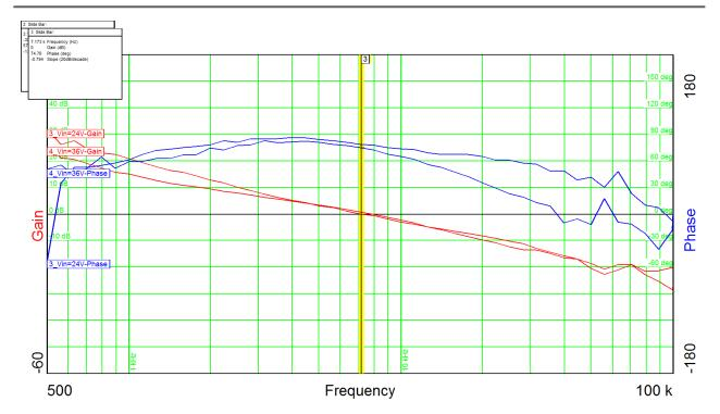
Output power = 51V@1.25AInput voltage = 24VDCPhase margin = 7.2kHz
