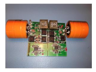
Input voltage = 36VDC Output power = 130W Ambient temperature = 25°C No heatsink, no airflow
