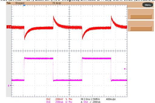
Ch2: Vout (200mV/div, 2ms/div, AC coupled, 20MHz BWL), Ch4: Iout (200mA/div)
