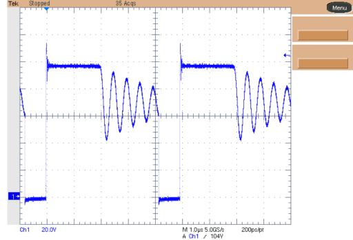
Ch1: Q1 drain Voltage (20V/div, 1us/div, No BWL), full load.
