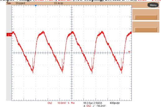
Ch.2: Output Voltage (20mV/div, 20us/div, AC coupling, 20MHz BWL), Iout = 100mA
