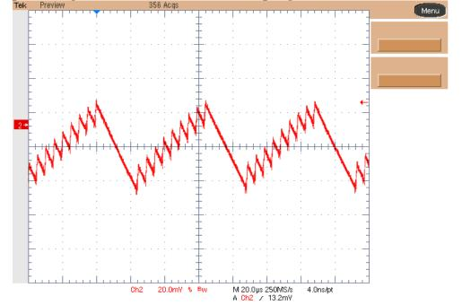
Ch.2: Output Voltage (10mV/div, 2us/div, AC coupling, 20MHz BWL), Iout = 500mA
