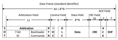
Figure 3. Standard CAN Frame Format
