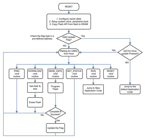
Figure 6. CAN Bootloader Flowchart
