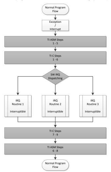
Figure 1. Program Flow With Common IRQ Handler
