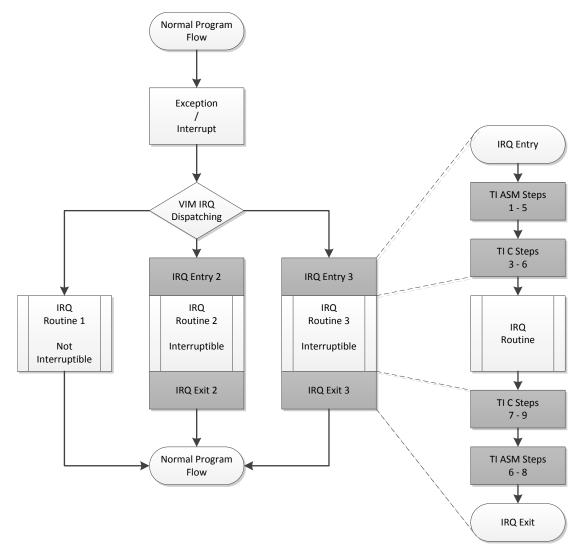
Figure 3. Program Flow With selective IRQ Wrappers
