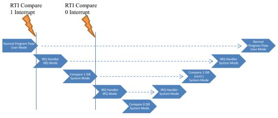
Figure 2. Example Application Program Flow
