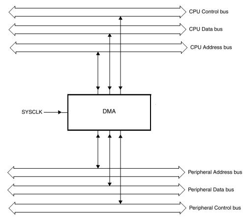
Figure 1. DMA Controller System Level Diagram
