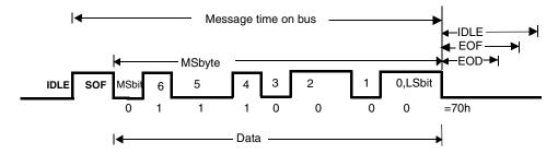
Figure 4. Typical C2SIa Data Frame Format Without In-Frame Response
