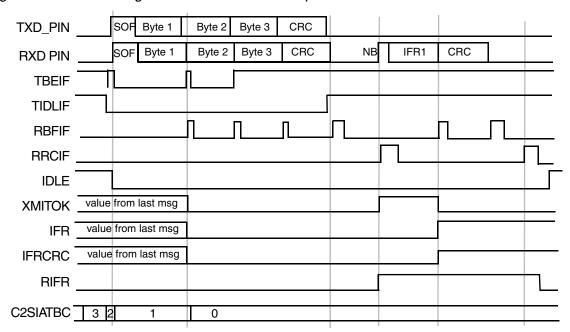
Figure 8. Send Message and Receive IFR Example
