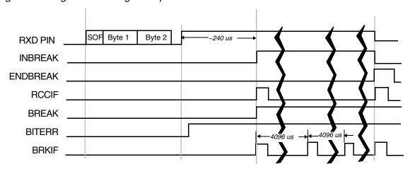
Figure 9. Long Break Timing Example
