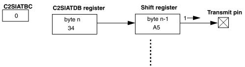
As soon as the shift register has completely shifted out byte n-1, byte n is loaded from the C2SIATDB register into the shift register. The C2SIATDB is now empty.
