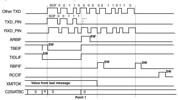
Figure 10. Loss of Arbitration Timing Example
