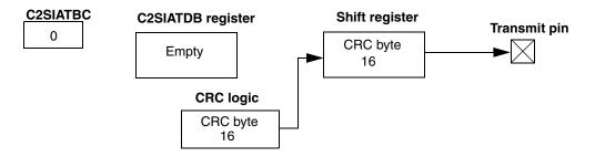
During transmission, the C2SIa's receiver and transmitter monitor each bit that the transmitter delivers to the C2SI bus to detect loss of arbitration. Since high voltage is the dominant level, arbitration is lost when the transmitter attempts to deliver a low voltage to the C2SI bus and the receiver detects a high voltage on the data link. This event forces the transmitter to immediately enter the idle state. It also causes the arbitration lost bit (ARBIF), transmit idle bit
