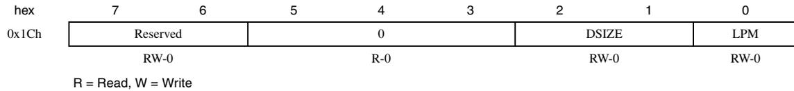
Table 10. EBM Control Register 1 (EBMCR1) Bit Descriptions
