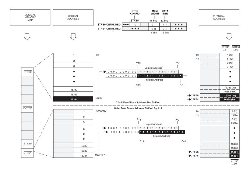
Figure 13. 16/8-Bit Memory Address Translation: Data Size > Memory Width
