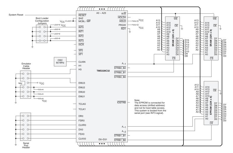
Figure 11. 16/8-Bit Memory Configuration: A Complete Minimum Design
