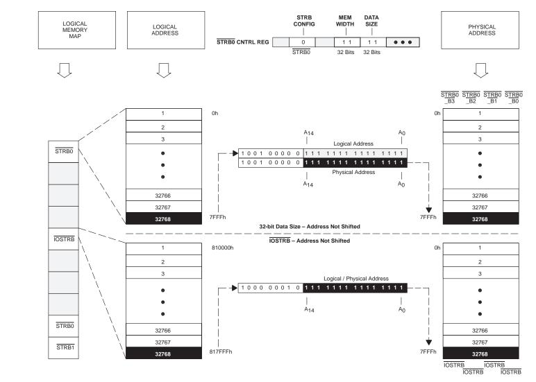
Figure 8. 32-Bit Memory Address Translation: Data Size = Memory Width
