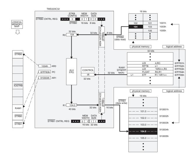
Figure 3. STRB0 and STRB1 Data Access: Data Size ≠ Memory Width
