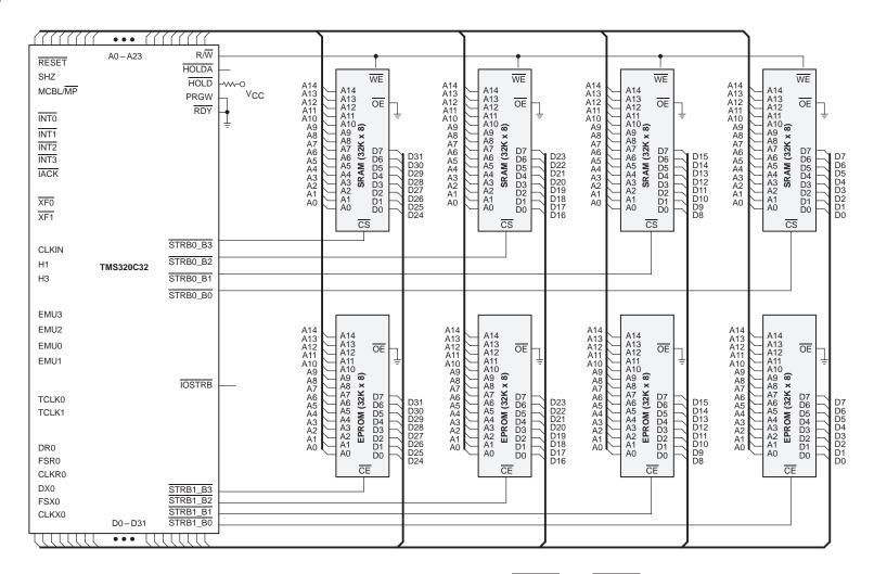
Figure 9. 32-Bit Memory Configuration (STRB0 and STRB1)
