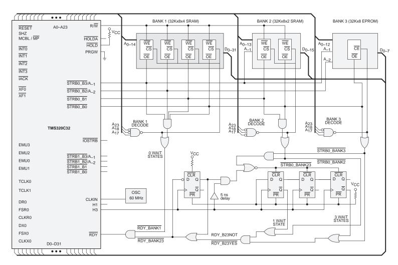
Figure 20. RDY Signal Generation for STRB0 Cycles
