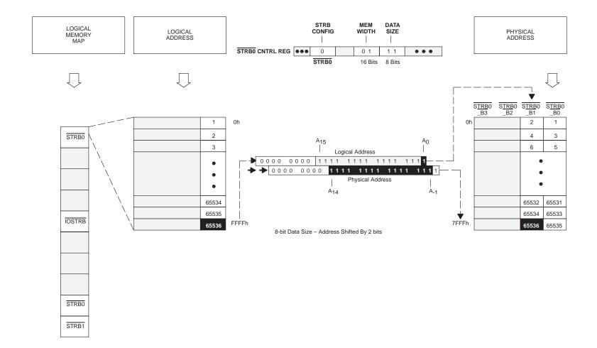
Figure 14. 16/8-Bit Memory Address Translation: Data Size < Memory Width
