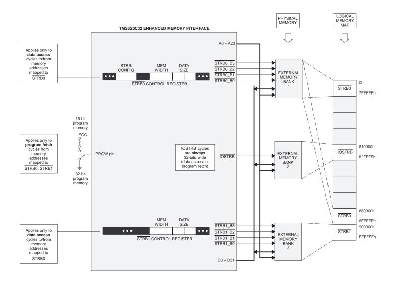
Figure 1. STRB0 and STRB1 Control Registers and the PRGW Pin
