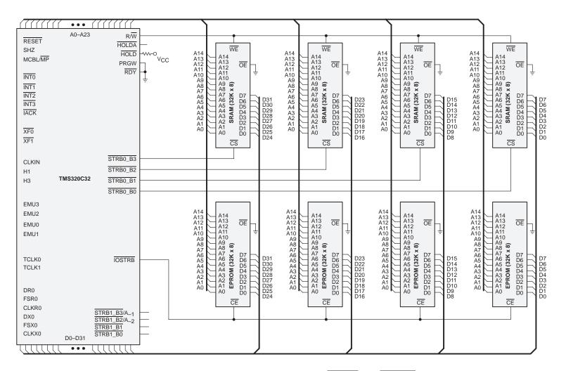
Figure 7. 32-Bit Memory Configuration (STRB0 and IOSTRB)
