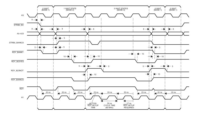
Figure 21. RDY Signal Generation Timing Waveforms
