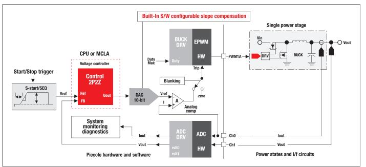
Fig. 4 –TI's new kits allow developers to jumpstart digital power designs, enabling and simplifying more complex power supply functions that are in high demand, such as Peak Current Mode Control (PCMC) with Slope Compensation, using no additional external circuitry.
