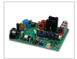
Fig. 2a – High Voltage 2-Phase Interleaved PFC
