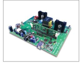
Fig. 3a –Isolated Phase-Shifted Full Bridge (PSFB) DC/DC Kit
