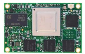
Figure 1. SolidRun's AM64x SoM Featuring AM6442. (Image Courtesy of SolidRun Ltd.)
