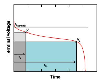
Figure 1. Typical Discharge Curve of a Single-cell Battery
