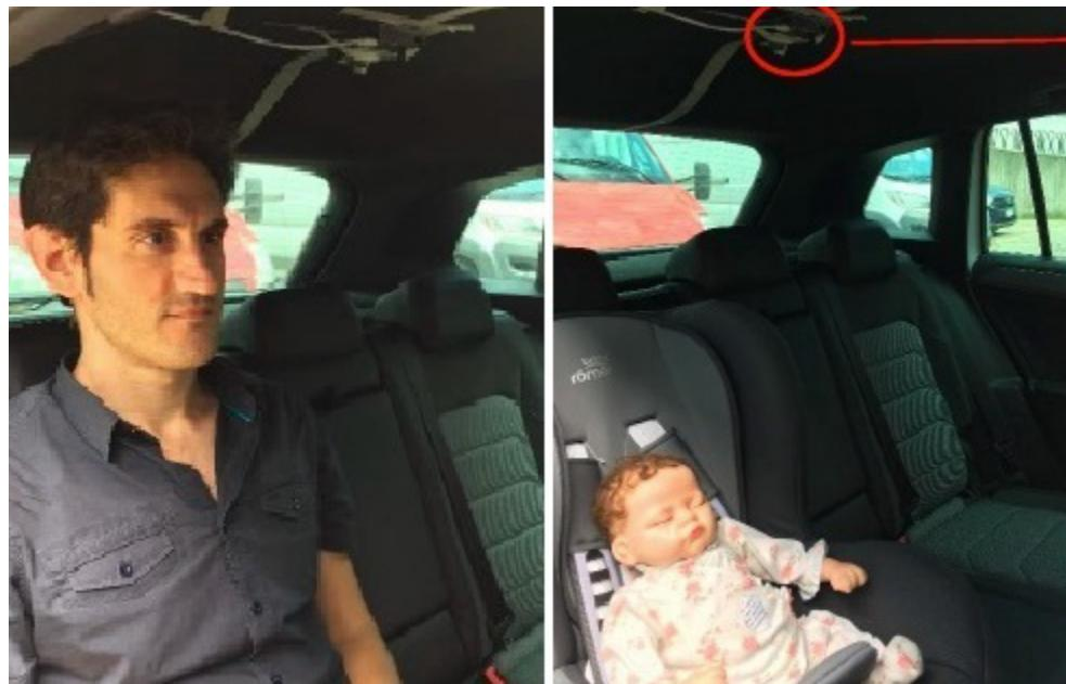
**Figure 3. Detecting and Distinguishing between an Adult and Child Occupant Using the AWR1843 Sensor Mounted on the Ceiling (Image Source: Azcom Technology)**
