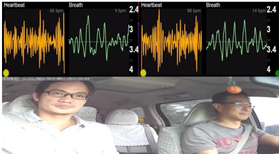
**Figure 1. Detecting Driver and Passenger Vital Signs Using the TI AWR1642 Sensor in a Moving Car**
