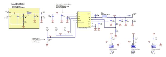
Figure 3. Schematic for EMI Filtering and LM53601-Q1 Power Supply
