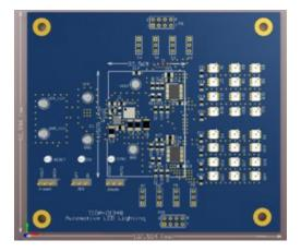
Figure 2. LED Automotive Reference Design
