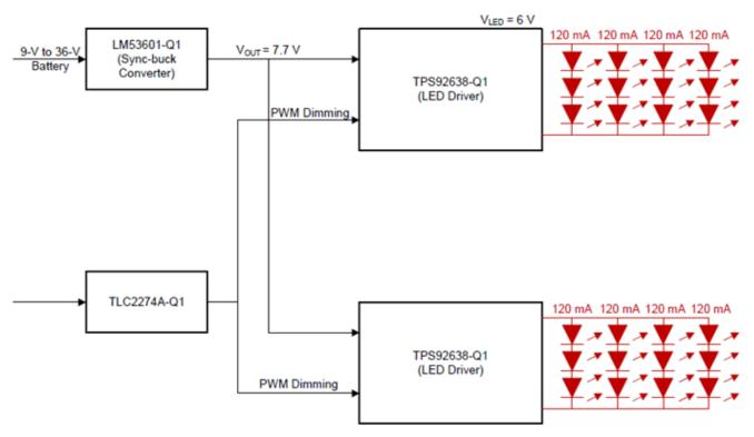
Figure 1. Automotive LED Power-supply Reference Design
