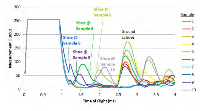
Figure 2. Example Ultrasonic Sensor Response During Kicking Gesture
