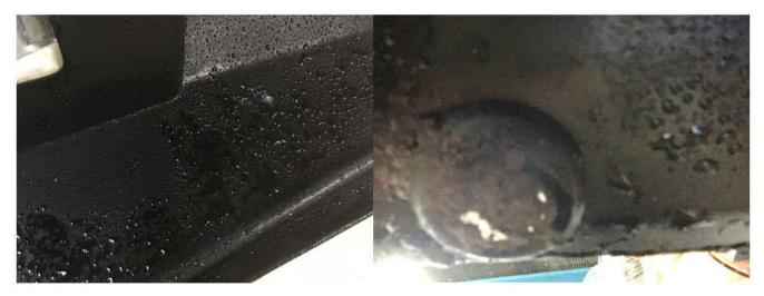
Figure 3. Water on Capacitive Sensor, and Mud on Ultrasonic Sensor
