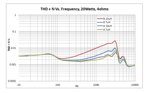
Figure 3. TPA3251D2EVM Plot of THD+N and Signal Frequency
