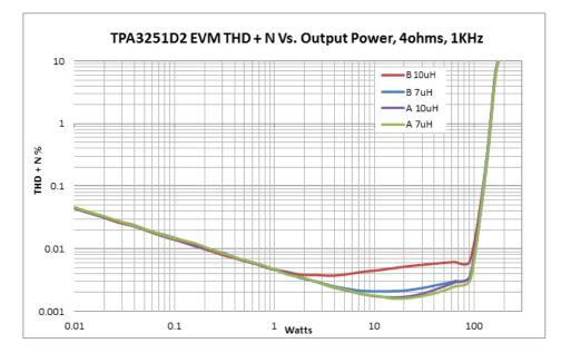
Figure 2. TPA3251D2EVM Plot of Output Power and THD+N for Measured Inductors
