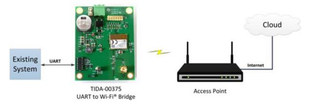
Figure 3. Wireless data connection to the cloud
