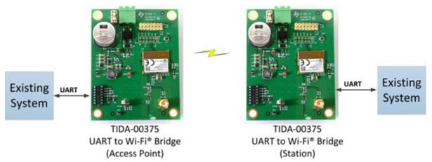
Figure 2. Wireless bridge using one TIDA-00375 as an access point
