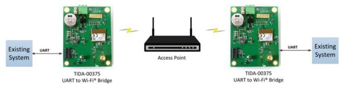
Figure 1. Wireless bridge over an existing Wi-Fi network
