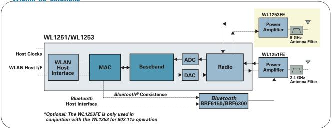
The WiLink 4.0 platform also includes support for Voice over WLAN (VoWLAN) applications which are driving WLAN adoption in mobile devices. As single-chip solutions with low cost, power and small size, the WL1251 and WL1253 WiLink 4.0 solutions are driving VoWLAN access into consumer cell phones. WiLink 4.0 solutions are VoWLAN-ready with support of:
