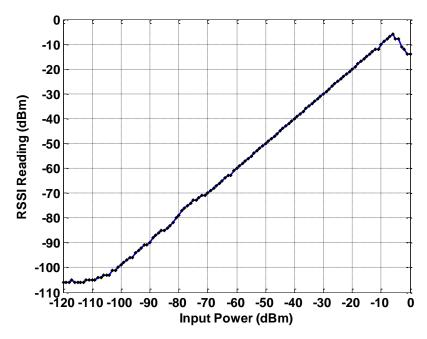
Figure 4.11. Typical RSSI vs. Input Power Level, LGM, 50 kbps
