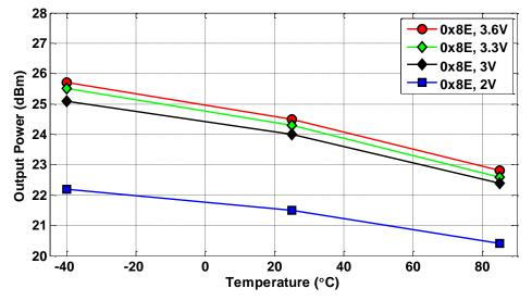
Figure 4.13. Typical Output Power vs. Temperature and Power Supply Voltage. PATABLE = 0x8E
