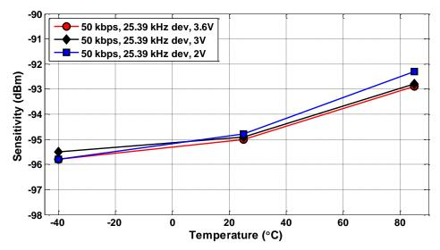
Figure 4.5. Typical Sensitivity vs. Temperature and Power Supply Voltage, LGM, 50 kbps
