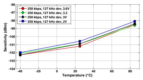
Figure 4.3. Typical Sensitivity vs. Temperature and Power Supply Voltage, HGM, 250 kbps
