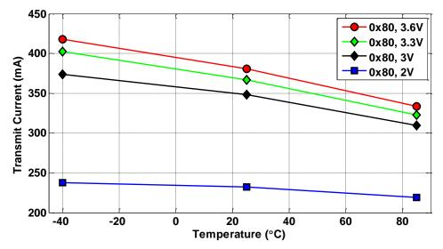
Figure 4.14. Typical TX Current Consumption vs. Temperature and Power Supply Voltage. PATABLE = 0x80
