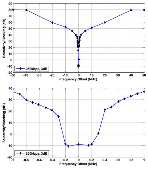
Figure 4.9: Typical Blocking / Selectivity, 250 kbps
