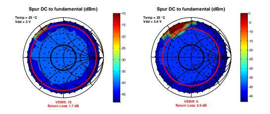
Figure 4.19. Spurious Frequency Components vs. Load Impedance at SMA Connector at 25°C. PATABLE = 0x80.
