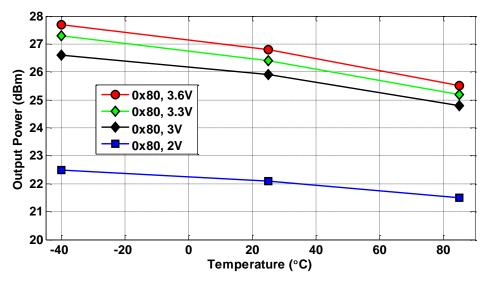
Figure 4.12. Typical Output Power vs. Temperature and Power Supply Voltage. PATABLE = 0x80
