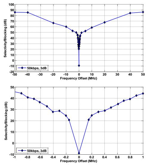
Figure 4.8. Typical Blocking / Selectivity, 50 kbps
