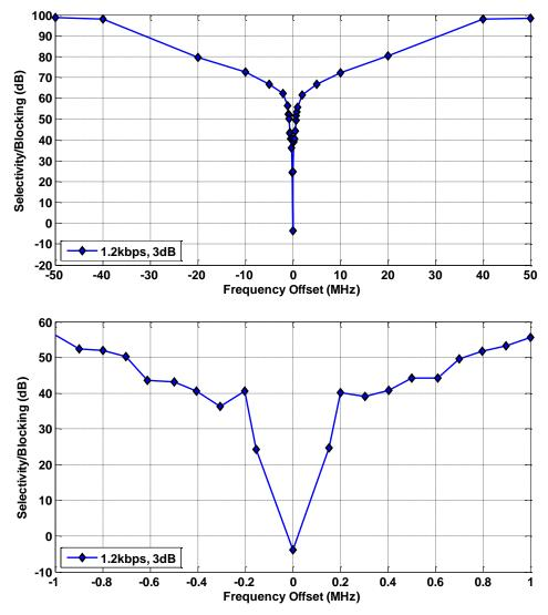
Figure 4.7. Typical Blocking / Selectivity, 1.2 kbps
