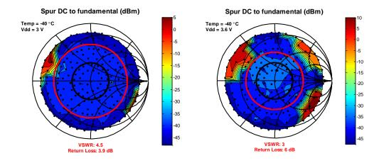
Figure 4.20. Spurious Frequency Components vs. Load Impedance at SMA Connector at -40°C. PATABLE = 0x80.
