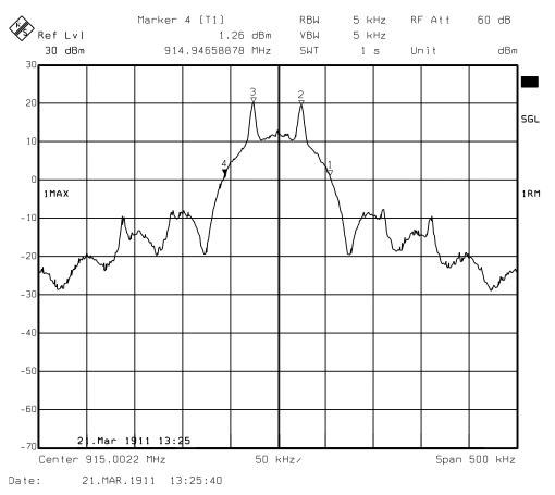
Figure 4.16. Typical Modulation Bandwidth, 50 kbps, PATABLE = 0x80. Measured according to FCC 15.247
