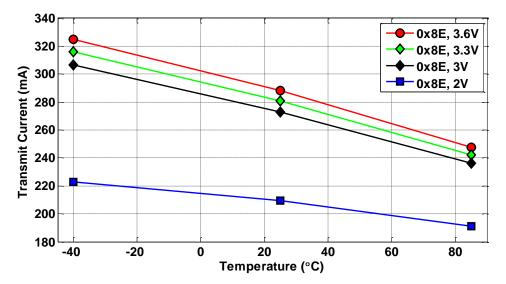
Figure 4.15. Typical TX Current Consumption vs. Temperature and Power Supply Voltage. PATABLE = 0x8E
