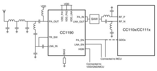
Figure 5.1. Simplified CC11xx-CC1190 Application Circuit
