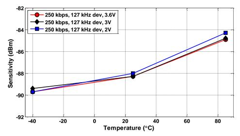
Figure 4.6. Typical Sensitivity vs. Temperature and Power Supply Voltage, LGM, 250 kbps
