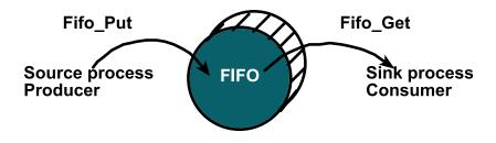
Figure 2. The FIFO is used to buffer data between the producer and consumer.
