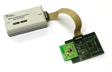
Figure 9 - EM and MCU board operating standalone
