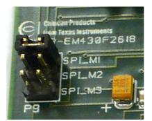
Figure 23 - SPI Mode selection header
