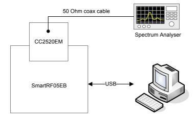
Figure 13 - Output power measurement set up
