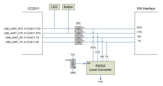
Figure 18 - UART RS232 signals and jumpers
