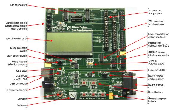
SmartRF05EB is the motherboard in the system, hosting all of the user interfaces and connections to external interfaces.
