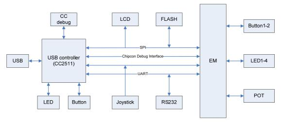
Figure 15 - SmartRF05EB architecture
