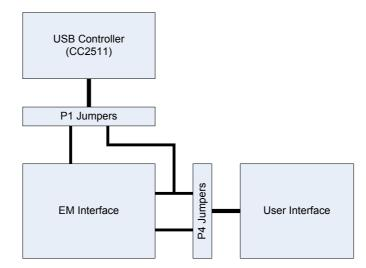
Figure 19 - Basic signal flow on the evaluation board
