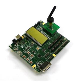
Figure 11 - CC2520EM connected to SmartRF05EB
