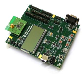
Figure 7 - CC2520EM and SmartRF05EB
