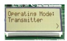
Select transmitter on one of the SmartRF05EB's and receiver on the other by navigating with the joystick. Confirm the selection by pressing Button 1 on both devices. The receiver is now ready to receive packets.
