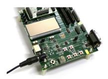
Alternatively a 4-10V DC power source using the jack connector can be applied. The centre pin is + and the sleeve is connected to ground. Set the power source jumper on the EB in position USB/DC.
