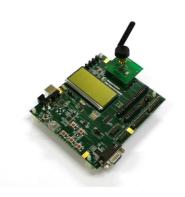
In order to use the SmartRF Studio the CC2520EM is connected directly to the SmartRf05EB.
