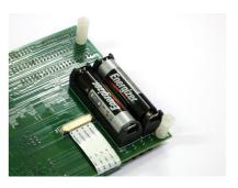
There are three different ways of applying power to the SmartRf05EB. The first method is to insert 2 AA batteries to the battery connectors underneath the board.
