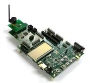
Insert a CCMSP-EM430F2618 into both the SmartRF05EB's. The connectors will only fit in one position. Connect antennas to both of the CC2520EM. Insert this board into the CCMSP-EM430F2618. These connectors will also fit in only one position. Do not force the boards.
