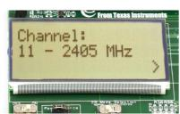
Select a channel between 11 and 26 (2405-2480 MHz). The channel is selected by navigating the joystick to the right or left. Confirm the selection by pressing Button 1.
