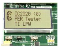
When power is applied to the board set the power switch in the ON position and the PER test program will start. The LCD will display the screen as shown in the picture above. Press Button 1 to enter the menu.
