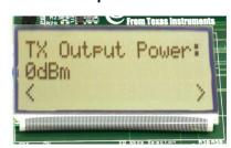
On the transmitter node, selection of TX output power and burst size (number of packets to send) is also needed. Select TX output power by navigating the joystick, either -4 dBm, 0 dBm or 4 dBm, and confirm with Button 1.
