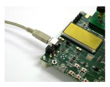
The SmartRf05EB can also be powered from the USB cable.
