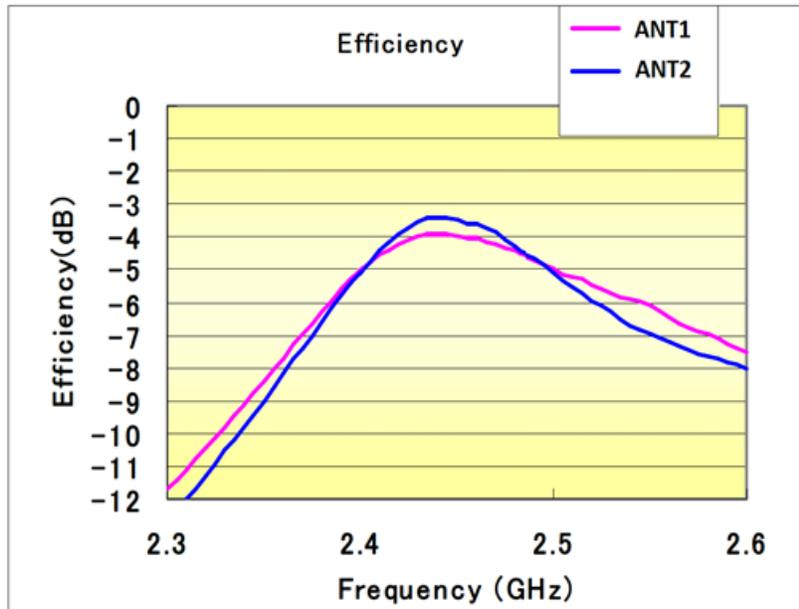
Figure 5. Antenna Efficiency
