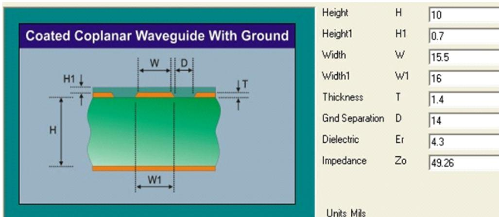
Figure 20. Trace Design for the PCB Layout
