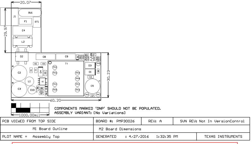
The reference design PMP30026 Rev-B has been built on PMP30026 Rev-A Board
