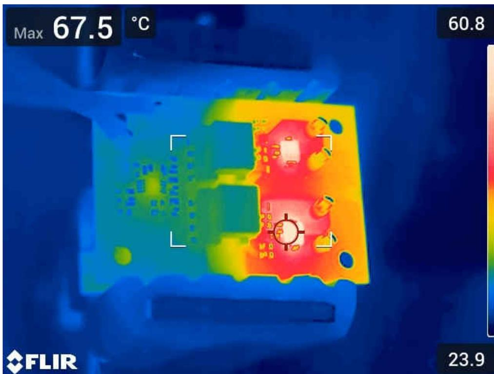
Figure 2-4. Thermal Image No Load
