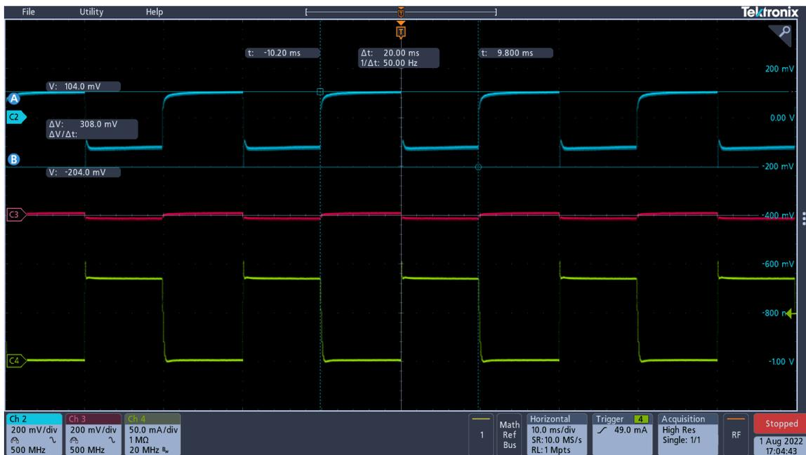
Channel 2 (blue) =  $V_{OUT2}$  AC coupled, Channel 3 (red) =  $V_{OUT1}$  AC coupled, Channel 4 (green) = load current of  $V_{OUT2}$
