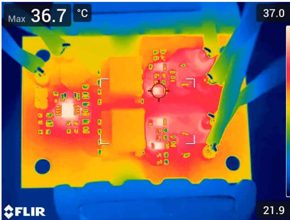
Figure 2-3. Thermal Image Full Load
