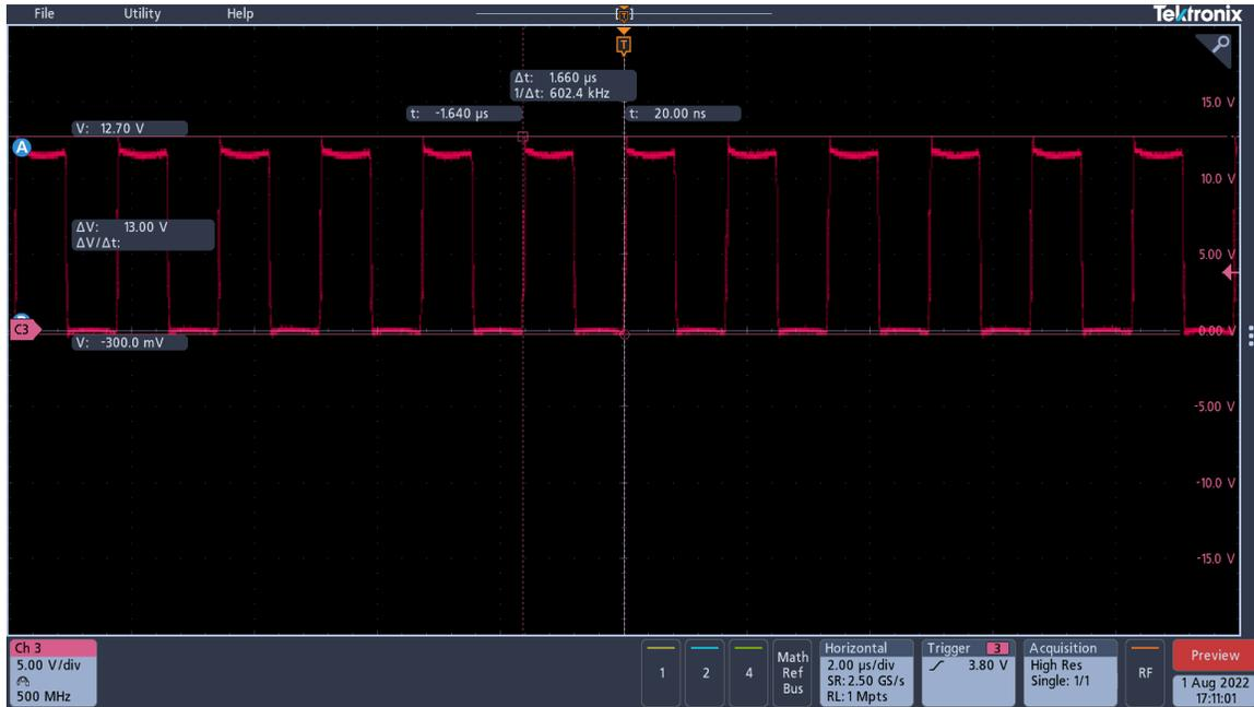
Figure 3-1. Switch Node Full Load
