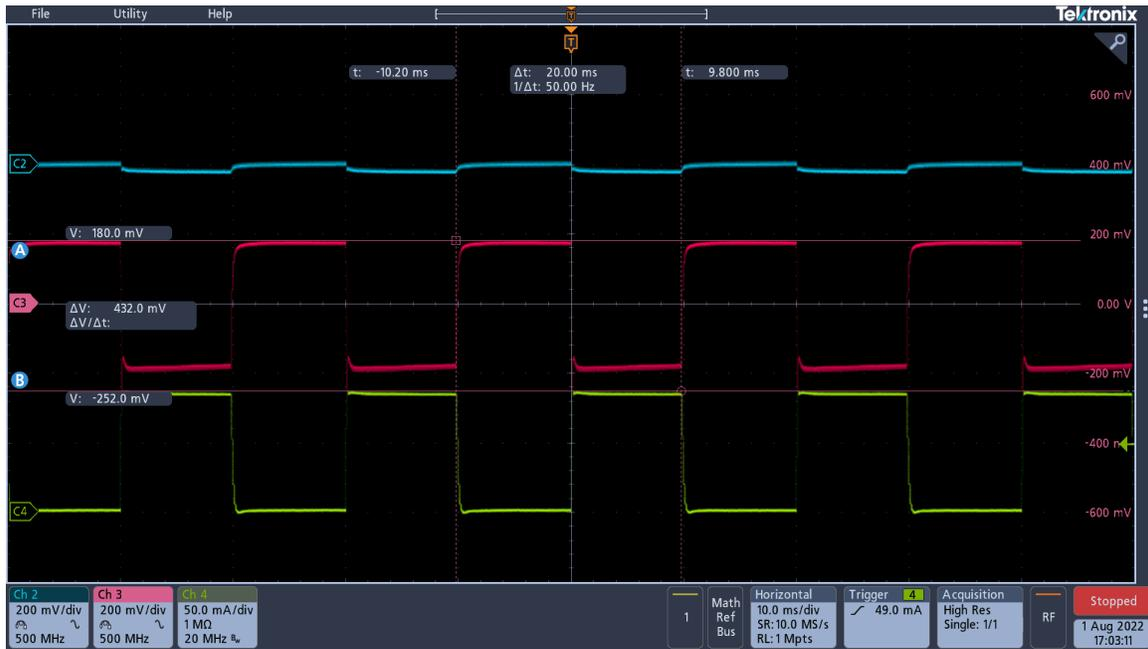
Channel 2 (blue) =  $V_{OUT2}$  AC coupled, Channel 3 (red) =  $V_{OUT1}$  AC coupled, Channel 4 (green) = load current of  $V_{OUT1}$
