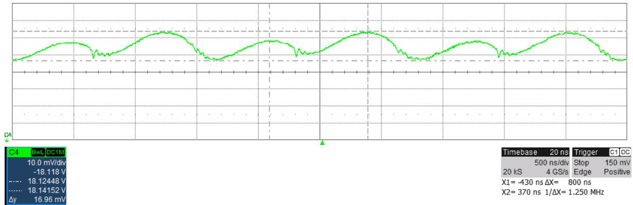
Figure 3-4.  $V_{OUT2}$  Output Ripple
