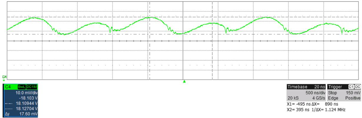
Figure 3-3.  $V_{OUT1}$  Output Ripple
