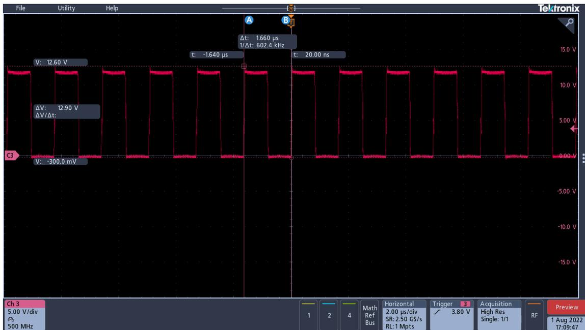
Figure 3-2. Switch Node No Load
