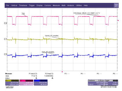
Figure 4. CHG Mode Ripple and Duty Cycle:  $V_{BUS} = 5 \text{ V}$ ,  $V_{BAT} = 3.7 \text{ V}$
