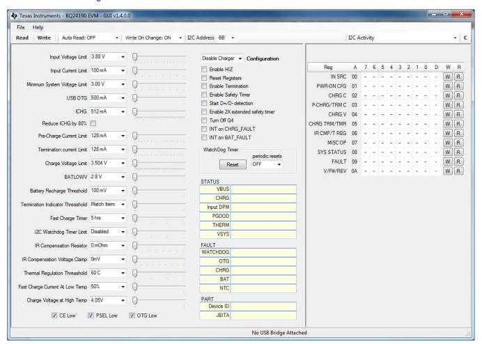
Figure 3. Main Window of the bq2419x Evaluation Software
