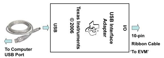
Figure 1. Connections of the HPA172 Kit
