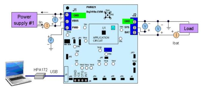
Figure 2. Original Test Setup for PWR021 (bq2419xEVM)
