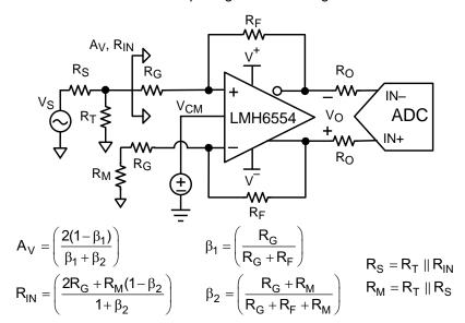
Figure 1. Single-Ended Input With Differential Output
