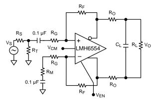
Figure 2. AC-Coupled Configuration
