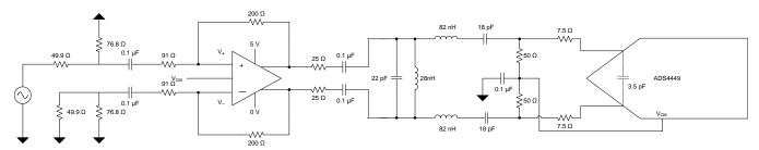
Figure 13. Circuit Used for the AC-Coupled Second Nyquist Zone Measurements
