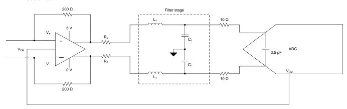
Figure 7. Typical Interface Circuit Driving an ADC
