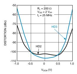
Figure 3. Distortion Versus Output Common-Mode voltage
