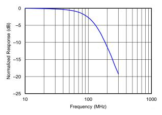
Figure 12. Normalized Gain Response — AC-Coupled First Nyquist Zone
