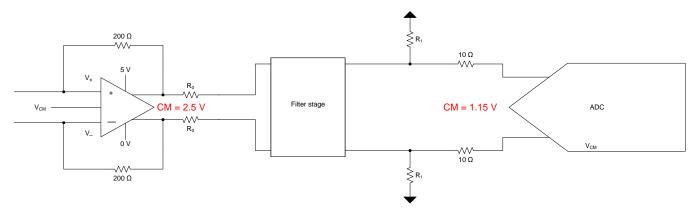
Figure 5. Interfacing With DC-Coupled Configuration
