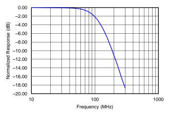
Figure 16. Normalized Gain Response — DC-Coupled First Nyquist Zone
