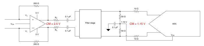
Figure 4. Interfacing With AC-Coupled Configuration
