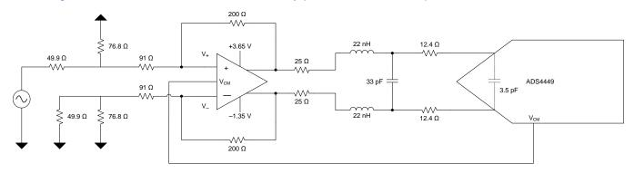
Figure 15. Circuit Used for the DC-Coupled First Nyquist Zone Measurements
