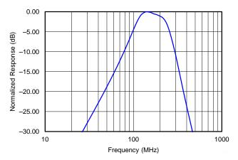
Figure 14. Normalized Gain Response — AC-Coupled Second Nyquist Zone
