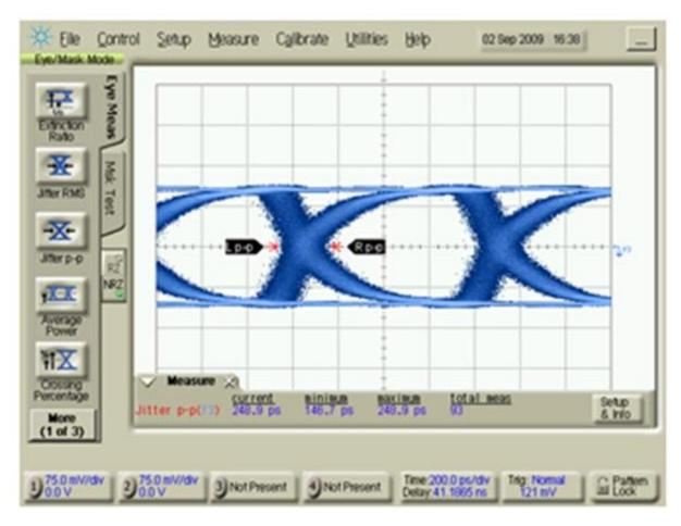
Figure 1. Eye diagram with PCLK = 43MHz, VODSEL = L
