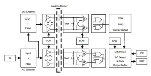
Figure 8. : ISO72x Isolator Internal Diagram
