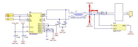
Figure 12. Isolated Transceiver
