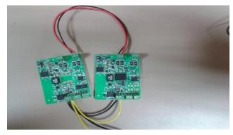
Figure 21. Two RS-485 Boards Daisy-Chained
