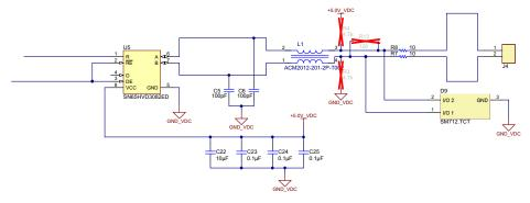
Figure 14. Half-Duplex Transceiver
