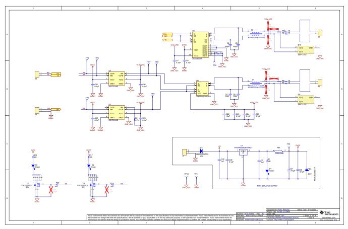
Figure 24. RS-485 Transceiver, Non-Isolated Power Supply
