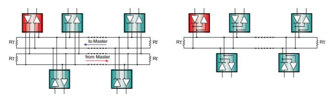
Figure 3. Full-duplex and Half-Duplex Bus Structures in RS-485
