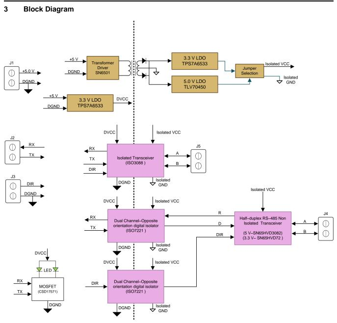
Figure 11. RS-485 Interface Module Block Diagram
