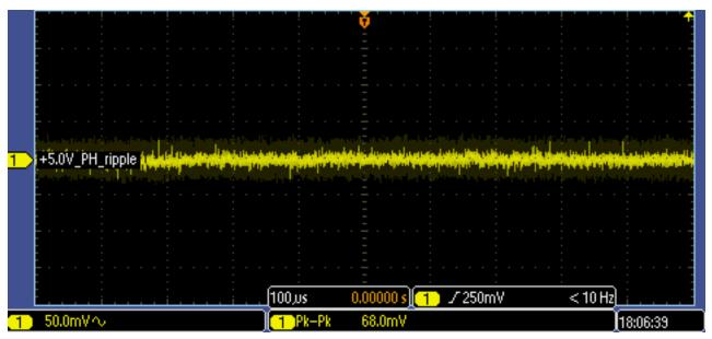
Figure 19. Ripple on +5.0V\_VDC
