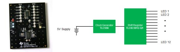
The design includes two modes of operation (ON and ROLLING) set by a jumper. ON operation sets each output to 5V. ROLLING operation cycles the state of the outputs sequentially.
