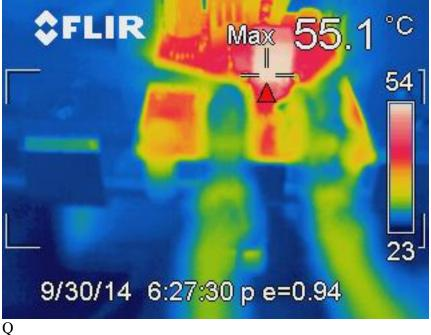
IR669: Inductor on top: 1V 15A and no fan
