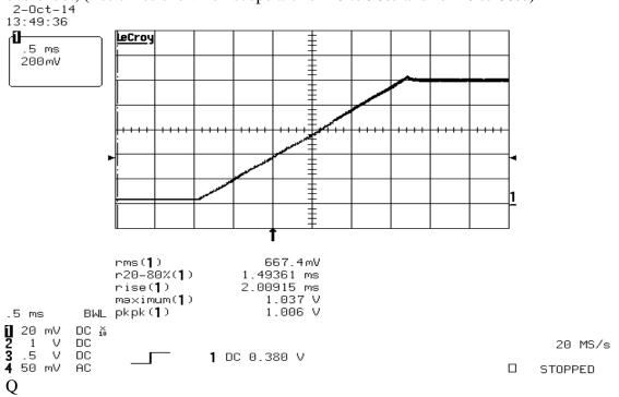
Start up at no load: with control pin going high: Rise time is  $\sim 2.55$  msec with  $\sim 30$  mV overshoot; (rise times shown on scope are for 10 to 90% and for 20 to 80%)
