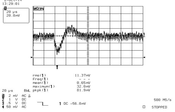
Step load response: 12Vin, 1.00Vout 11 to 26A in 4usec (0 to 15A in 4 usec had same undershoot). This also shows near full load ripple of about 20mV p-p.  $_{2-Oct-14}$
