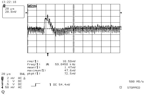
Details of step load across 20mOhms R18 tied to Vout: ~300mV (or 15A) in 3-4 usec. Scope ground on Vout side of R18, hence negative going voltage corresponds to current at 1A per 20mV.
