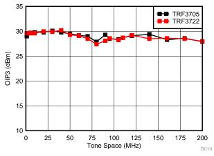
Figure 12. OIP3 versus Tone Spacing
