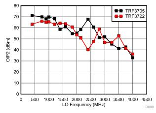
Figure 13. OIP2 versus LO Frequency
