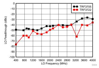
Figure 5. Unadjusted LO Feedthrough versus LO Frequency
