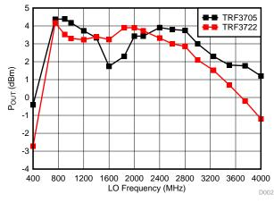
Figure 3. Output Power versus LO Frequency
