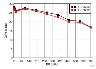
Figure 11. OIP3 versus Baseband Frequency
