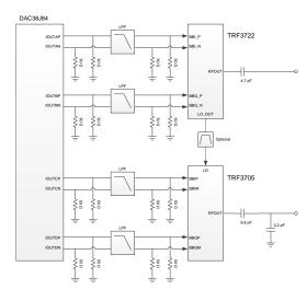
Wideband Dual Transmit Solution With Integrated Local Oscillator
