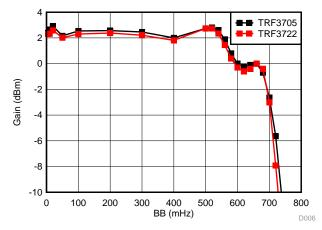
Figure 4. Output Power versus Baseband Frequency
