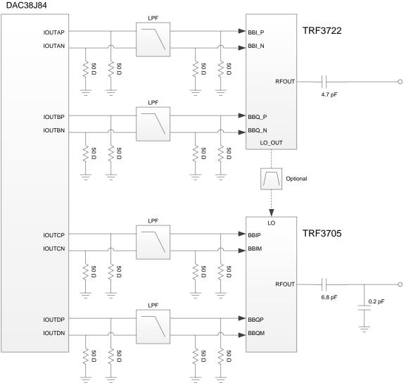
Figure 1. TSW38J84 Block Diagram
