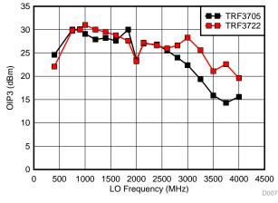
Figure 10. OIP3 versus LO Frequency
