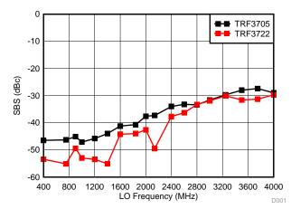
Figure 8. Unadjusted SBS versus LO Frequency
