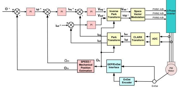
Figure 4. Block Diagram of Sensored FOC
