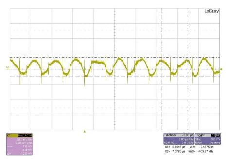
Output voltage ripple = 12.0mV
