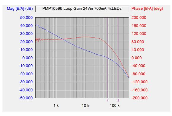
Figure 16 Closed loop response at 24Vin, 700mA, 4x LEDs
