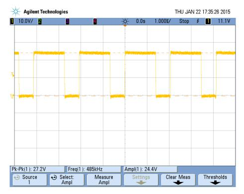
Figure 9 Switching waveform at 24Vin, 700mA, 4x LEDs
