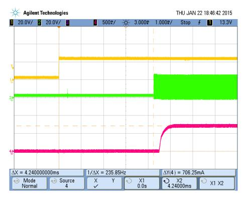
Figure 8 Start up at 24Vin, 700mA, 4x LEDs
