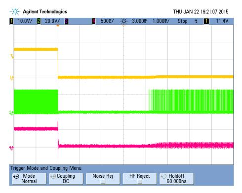
Figure 15 Short circuit test from 24Vin, 700mA, 4x LEDs
