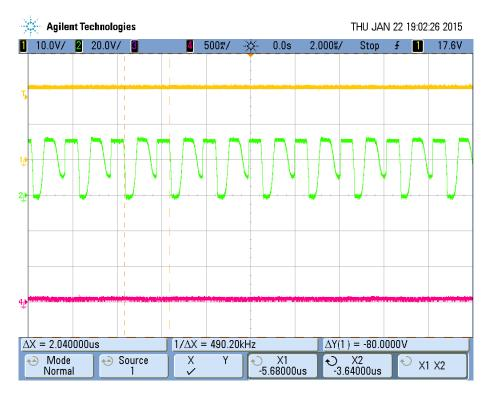
Figure 14 Open circuit operation at 30Vin
