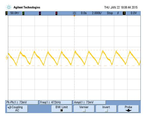
Figure 12 Input ripple at 24Vin, 700mA, 4x LEDs
