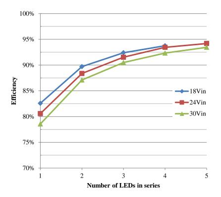
Figure 3 Power efficiency at 700mA output
