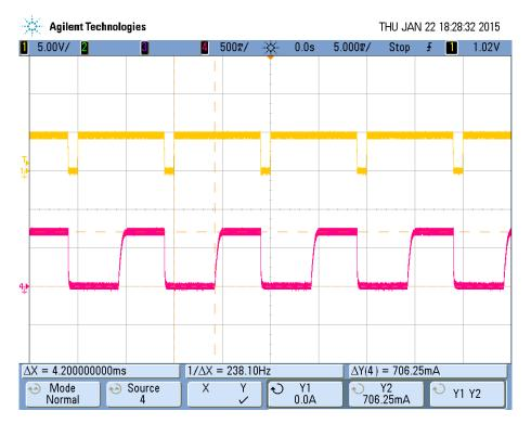
Figure 7 PWM at 90% duty cycle, average output current at 0.32A
