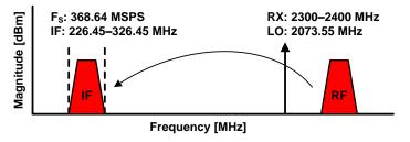
Figure 2. Frequency Plan for 3GPP Band 40
