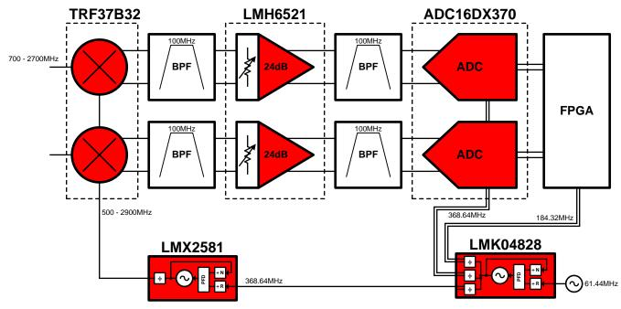
Figure 1. TSW16DX370EVM Block Diagram
