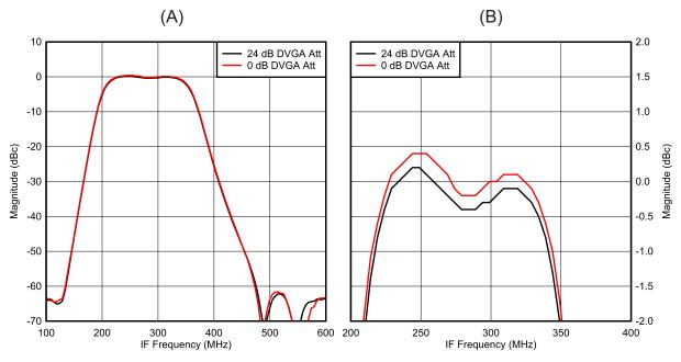
Figure 4. TSW16DX370EVM Selectivity Ch.A—Total Selectivity of IF Sub-System (A) and (B)
