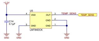
Figure 11. Heat Sink Temperature Sensor
