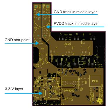
Figure 49. Layout Considerations for Power Handling and GND Tracks
