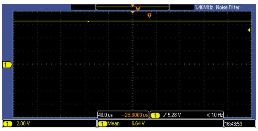
Figure 27. Voltage at AVDD Pin of DRV8303
