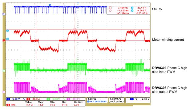
Figure 40. Cycle-by-Cycle Current Limiting When Motor is Medium Overloaded
