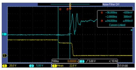
Figure 32. Dead Time Inserted by DRV8303 Measured at Rising Edge of Lower FET PWM
