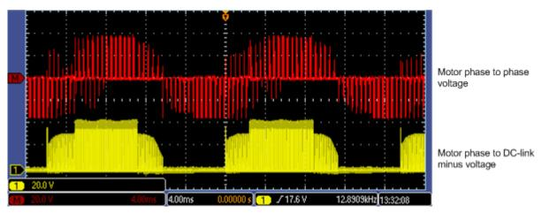
Figure 33. Phase-to-Phase Voltage at Motor Winding Terminals
