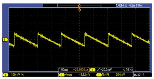
Figure 24. Ripple at GVDD Pin Voltage of DRV8303
