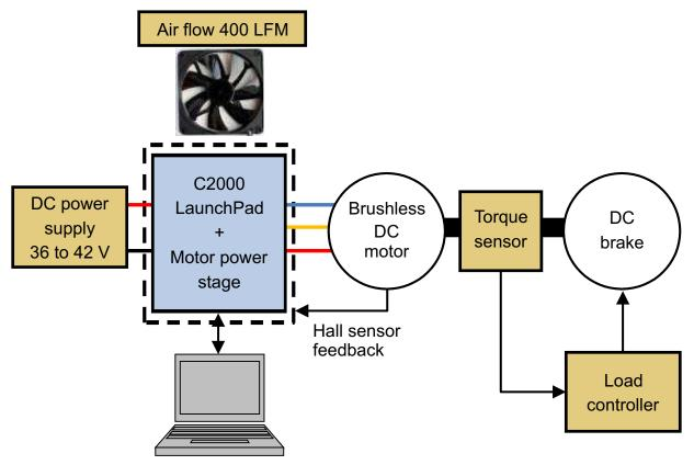
Figure 34. Block Diagram of Load Test Setup
