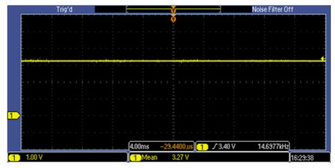
Figure 21. Output Voltage of 3.3 V from Step-Down Converter
