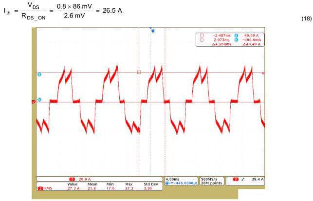
Figure 36. Motor Winding Current Loaded on Test Setup
