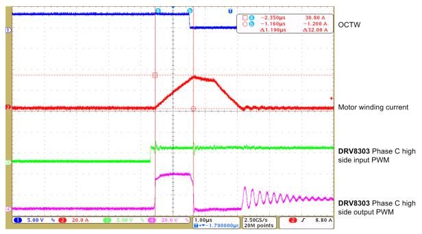
Figure 46. Cycle-by-Cycle Response Time
