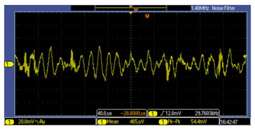
Figure 28. Ripple at AVDD Pin Voltage of DRV8303
