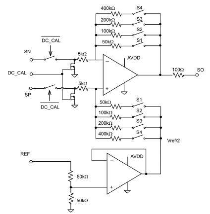
Figure 8. Simplified Block Diagram of Current Shunt Amplifier in DRV8303
