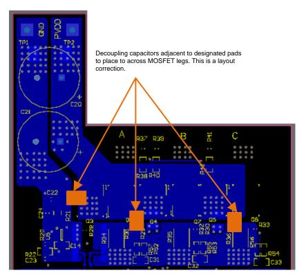
Figure 50. Mounting of Decoupling Capacitors for Inverter Legs
