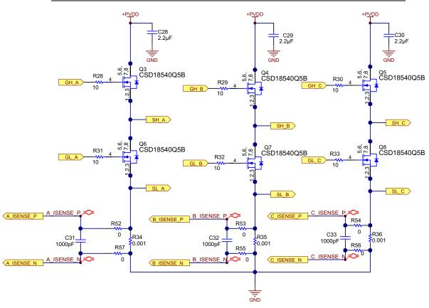
Figure 6. Three-Phase Inverter of Power Stage
