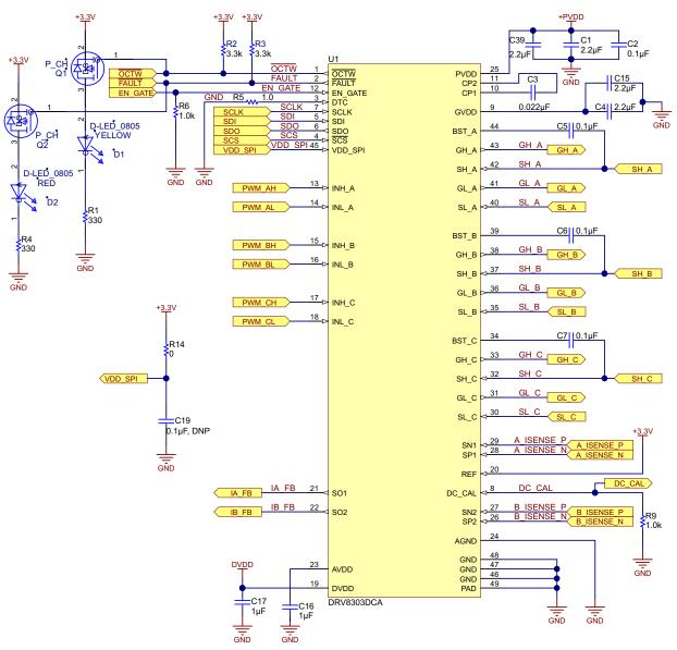
Figure 7. DRV8303 Schematic
