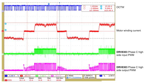
Figure 41 shows the motor heavily overloaded and the cycle-by-cycle is triggered almost every PWM cycle.
