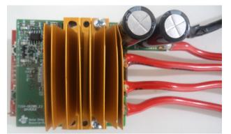
Figure 20. Assembled Power Stage With Heat Sink Mounting
