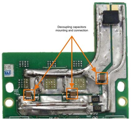
Figure 51. Mounting of Decoupling Capacitors for Inverter Legs
