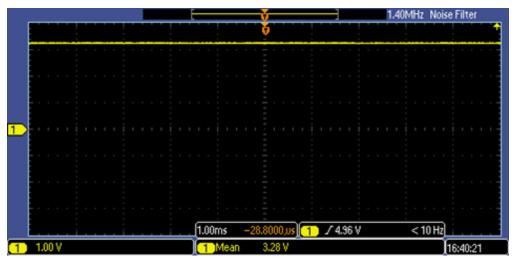
Figure 25. Voltage at DVDD Pin of DRV8303
