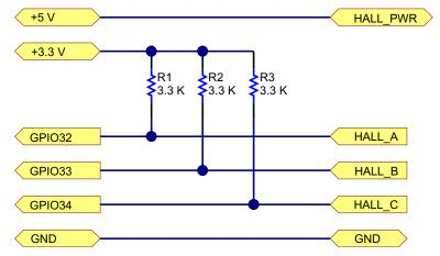
Figure 14. Hall Sensor Interface to LAUNCHXL-F28027 LaunchPad
