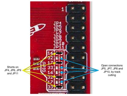
Figure 16. Jumper Modification on C2000 LaunchPad
