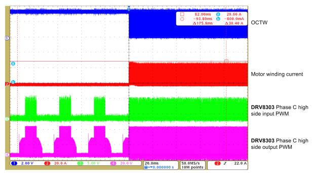
Figure 44. Motor Terminals Short Circuit Waveforms
