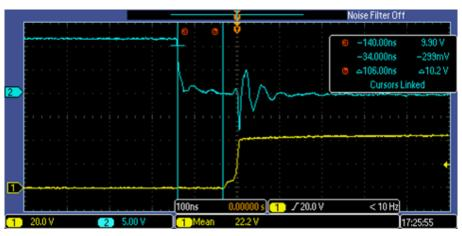
Figure 31. Dead Time Inserted by DRV8303 Measured at Falling Edge of Lower FET PWM
