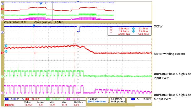
Figure 39. Cycle-by-Cycle Current Limiting When Motor is Lightly Overloaded (Zoomed View)
