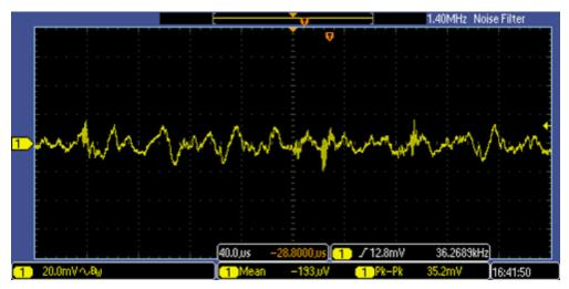
Figure 26. Ripple at DVDD Pin Voltage of DRV8303
