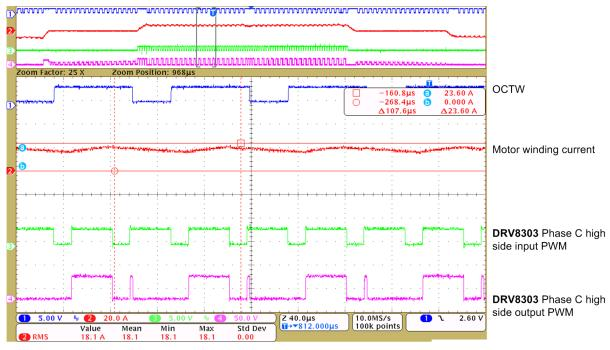
Figure 42. Cycle-by-Cycle Current Limiting When Motor is Heavily Overloaded (Zoomed View)
