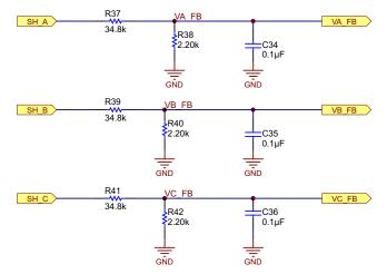
Figure 9. Motor Winding Voltage Sense Circuit
