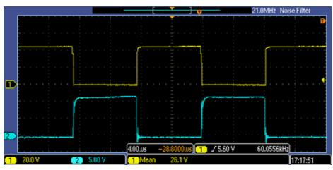
Figure 30. Complimentary PWM Gate Signal From DRV8303
