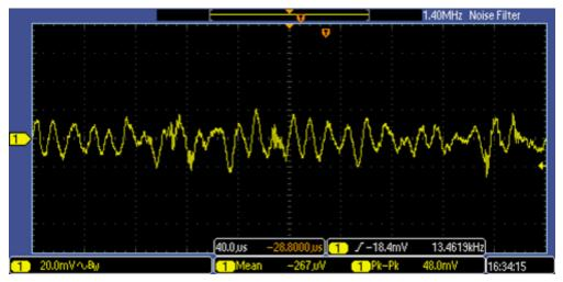
Figure 22. Ripple in 3.3-V Output from Step-Down Converter
