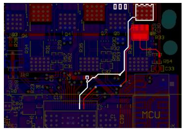
Figure 48. Differential Line for  $V_{\mbox{\tiny DS}}$  Sensing of MOSFETs
