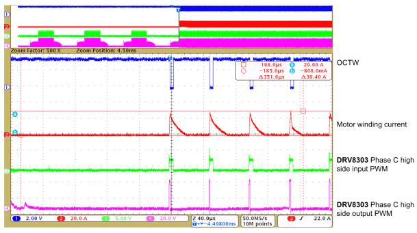
Figure 45. Motor Terminals Short Circuit Waveforms (Zoomed View)
