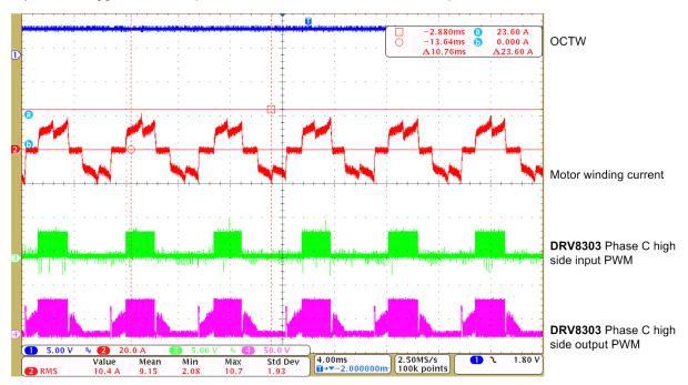
Figure 37. Motor Current Before Cycle-by-Cycle
