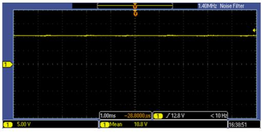
Figure 23. Voltage at GVDD Pin of DRV8303
