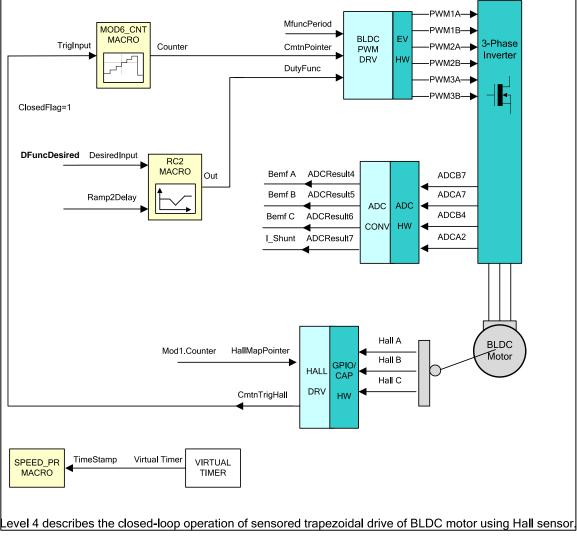
Figure 15. Level 4 Incremental System Build Block Diagram
