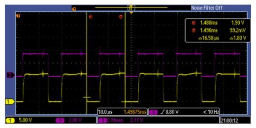
Figure 29. Low-Side PWM Input and Output of DRV8303
