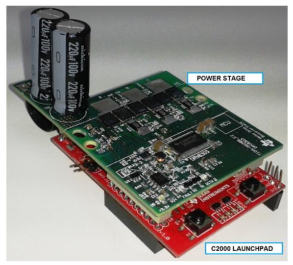
Figure 3. Assembled Power Stage Mounted With LaunchPad
