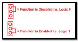
Figure 3 Three Pin Header Legend
