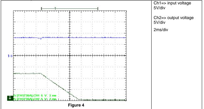
The shutdown waveform is shown in the Figure 5. The input voltage was set at 12V, with 1A load on the output.
