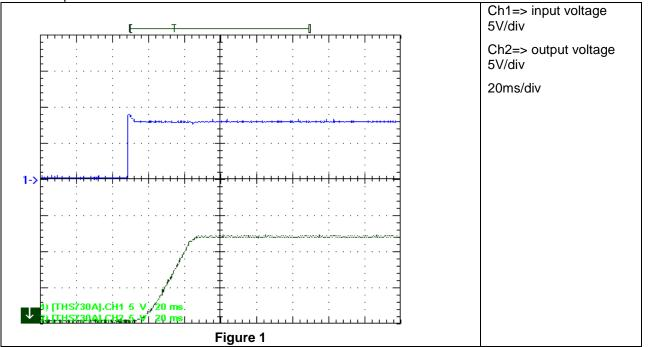
The startup waveform is shown in the Figure 2. The input voltage was set at 12V, with 1A load at the output.
