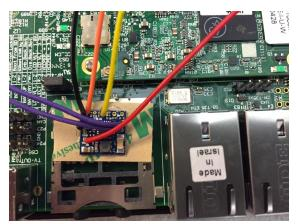
Figure 48. DRV2667EVM-MINI Board Connections
