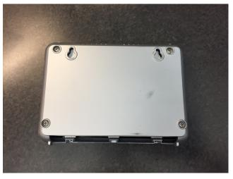
Figure 46. Enclosure with Back Cover Attached
