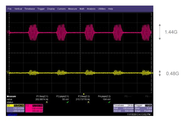
Figure 23. Acceleration Measurements for Piezos—Top Placement
