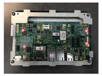
Figure 43. Motherboard and Carrier Frame Screw Locations
