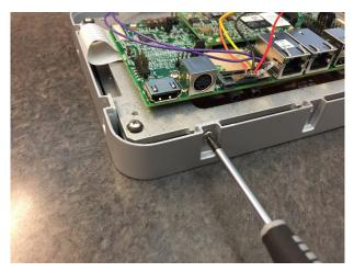
Figure 45. Secure Chassis to Carrier Frame
