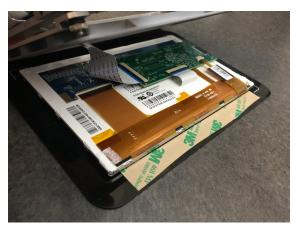
Figure 42. Tape on Backside of Touch Screen
