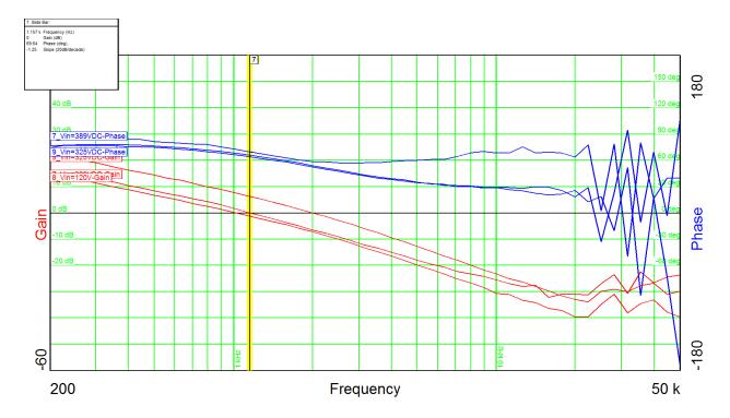
$\begin{array}{lll} \text{Output power} & = 30 \text{W} \\ \text{Input voltage} & = 120 \text{VDC} \\ \text{Phase margin} & = 68^{\circ} \\ \text{Bandwidth} & = 1.0 \text{kHz} \end{array}$
