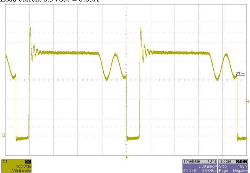
Input voltage = 85VDC Load current 12Vout = 2.5A Load current 8.5Vout = 0.05A
