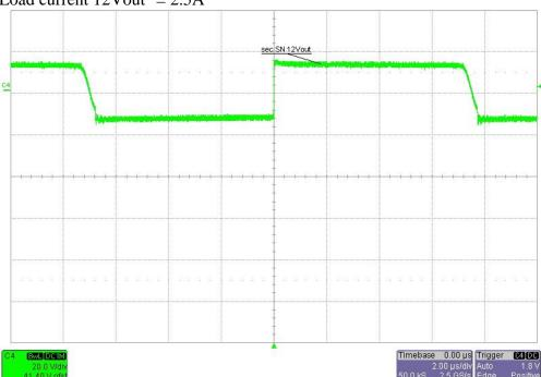
Input voltage = 390 VDCLoad current 12Vout = 2.5A
