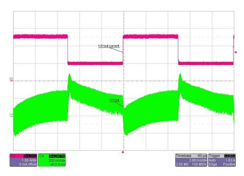
Input voltage = 230VAC Load current 12Vout = 1Ato2.5A
