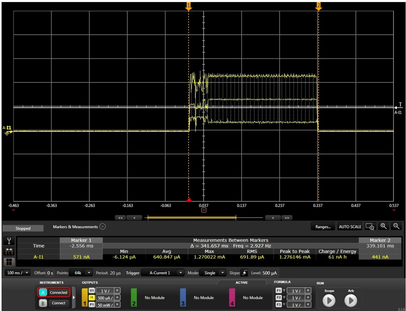
Figure 14. Power (in Milliwatts) During Active 1-Wire Operation
