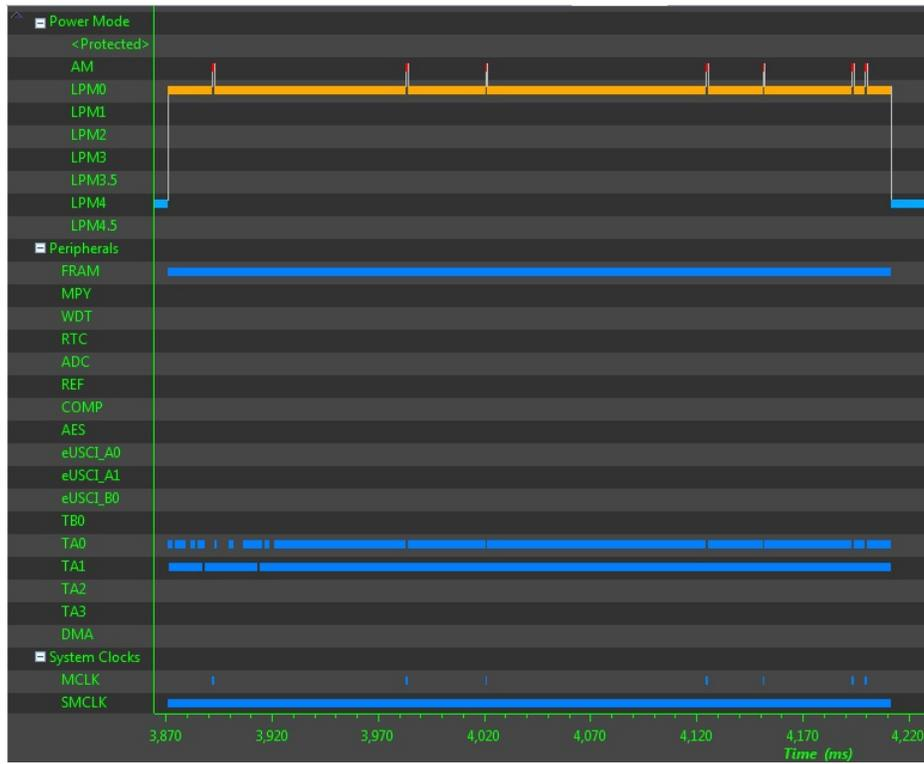
Figure 16. CPU and Peripheral States During Active 1-Wire Operation
