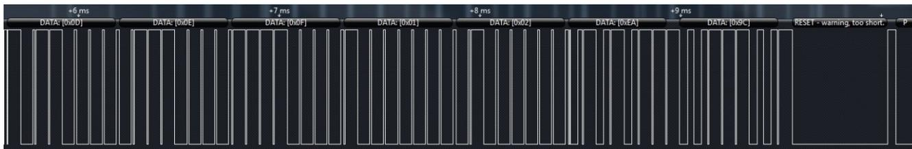
Figure 10. Write Scratchpad Example With CRC16 Response
