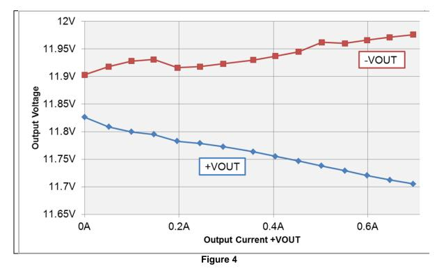
Deviation on load of negative rail <100mV, less than 1% Deviation of positive rail around 120mV, roughly 1%
