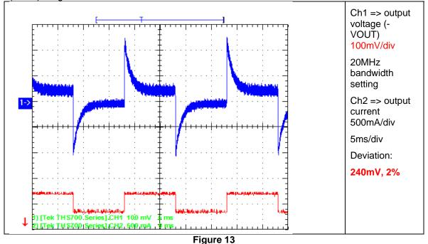
The Figure 14 shows the response to load transients. The load is switching from 0.35A to 0.7A (50 Hz). Positive VOUT was measured
