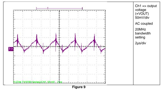
Output ripple around 100mVpp, so less than 1% of output voltage.
