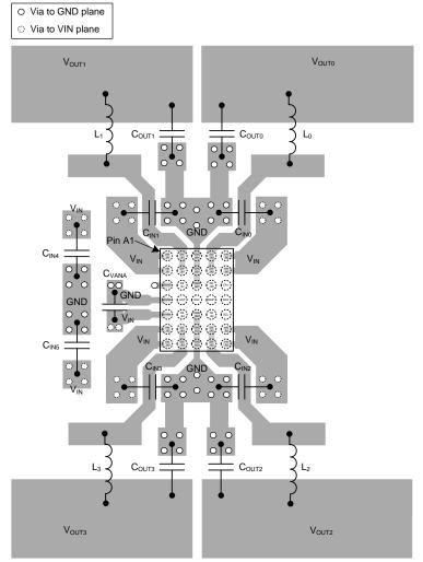
Figure 3: PCB layout example for LP8758-E0
