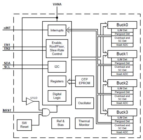
Figure 2: LP8758 Functional Block Diagram
