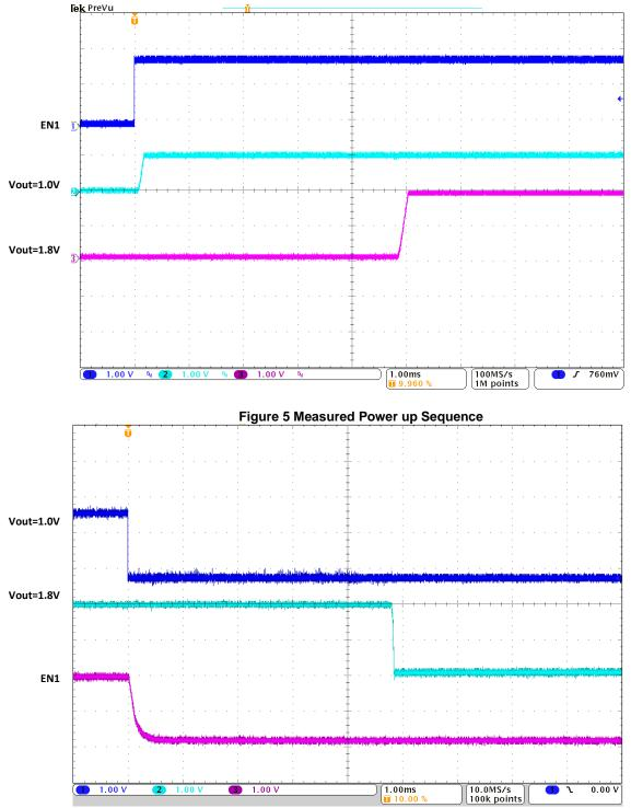
Figure 6 Measured Power down Sequence
